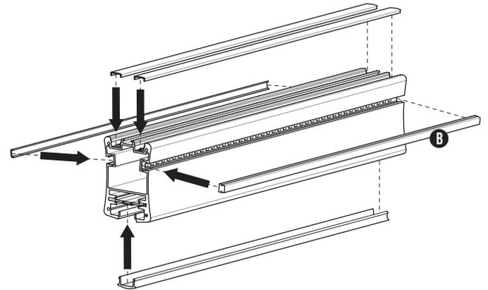
5. Slide in the suspension brackets, then tighten the bolts.
